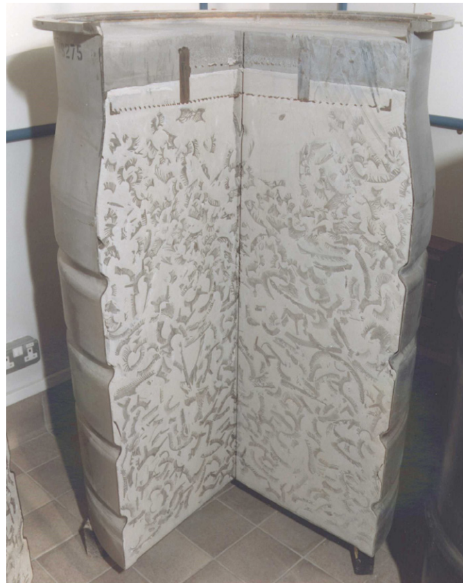
Figure 4 – Cut away of a replica 500L drum showing waste material encapsulated in grout. It should be noted that in this example the waste is evenly distributed within the grout, whereas normally the waste tends to settle towards the bottom of the drum
